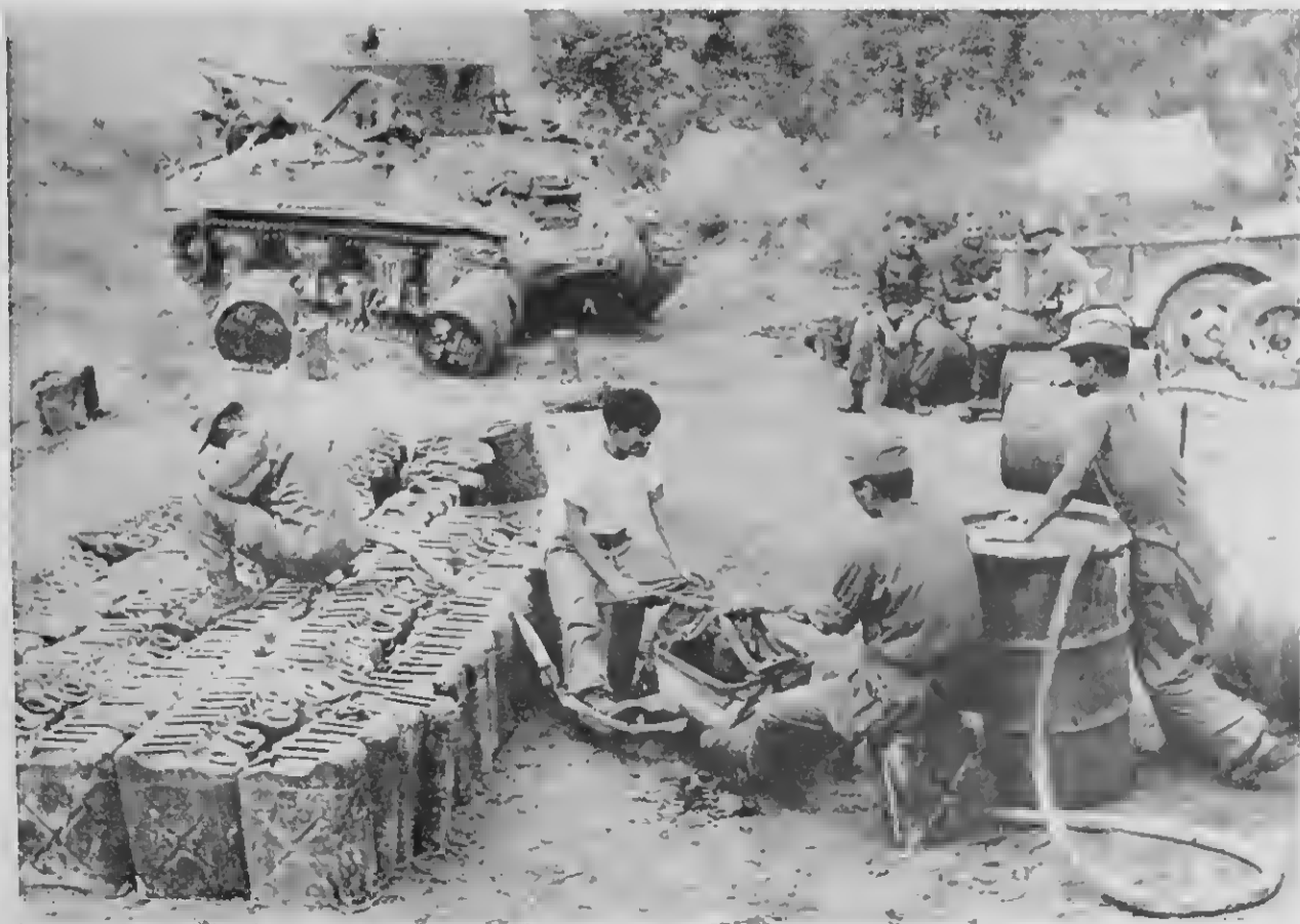
Hand-operated pump used to transfer gasoline from 55-gallon storage drums to the 5-gallon GI gas cans carried by UN tanks as fuel reserve.
